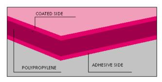
laminating roll is between 100°C and 115°C (to be checked according to lamination conditions).
