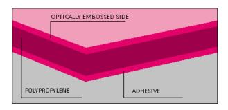
the result of preliminary tests. The optimum processing temperature of the laminating roll is between 100°C and 115°C (to be checked according to lamination conditions).
